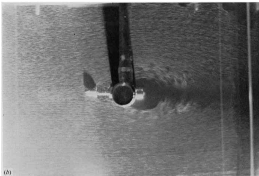
FIGURE 2. Hydrogen-bubble pictures, jet directed downstream. (a) No injection, R_D \cong 10^3 . (b) With 5% injection ratio, R_D \cong 10^3 .
